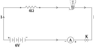
An electric lamp connected in series with a resistor of 4  $\Omega$  to a 6 V battery
