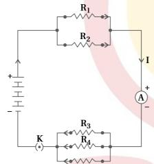
An electric circuit showing the combination of series and parallel resistors
