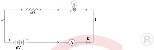
An electric lamp connected in series with a resistor of 4  $\Omega$  to a 6 V battery
