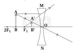
Object position: Between infinite point and optical centre
